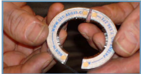
Equal proportions of epoxy and activator were then mixed, and small amounts were applied to the back of the ring.
