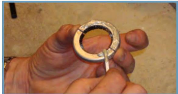
Prior to installing the ring, a narrow band of AEGIS® colloidal silver coating was applied around the shaft where the fibers contact it, to improve the surface conductivity. The ring was then installed on the shaft and re-taped.
