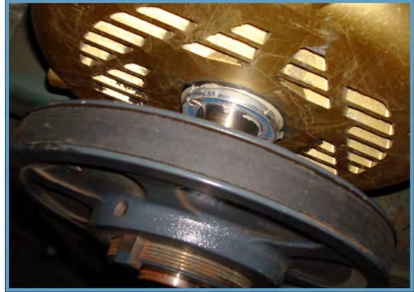
A hand-held heater was used to speed the epoxy's cure, and about half an hour after installation the shaft voltage was measured again. This time the reading was only 380 millivolts peak-to-peak.
