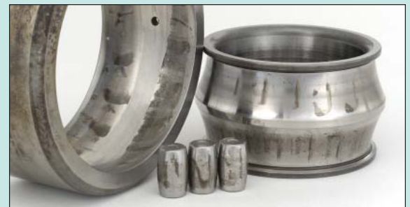
Fig. 15 Rust on Spherical Roller Bearing Caused by Water Ingress
