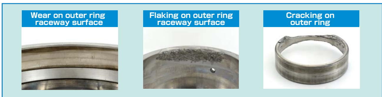
Fig. 3 Typical failure to Spherical Roller Bearings Supporting the Rolls of Continuous Casting Machines
