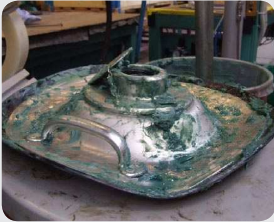
Figure 3: Dirty grease pump follower plate.
