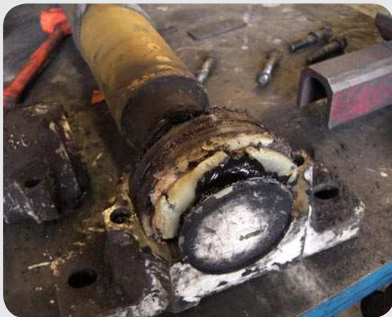
Figure 12 & 13: Housing overfilled. No grease drainage.
