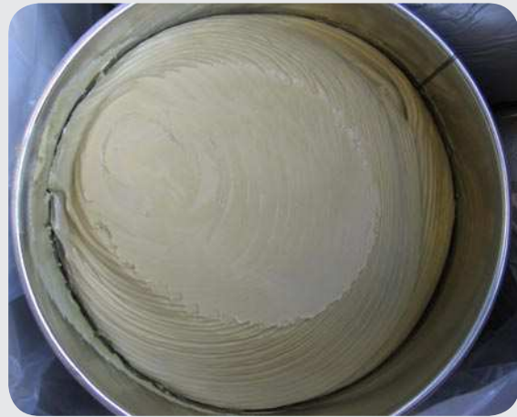
Figure 2: Grease stored for long time (Grease hardening)
