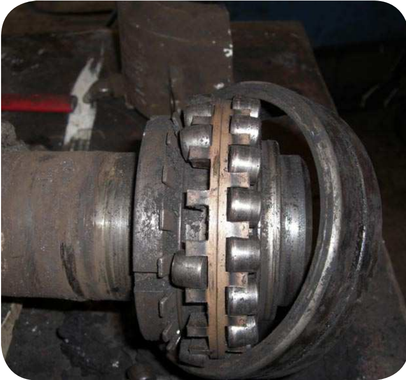
Figure 14: Undergreasing: Bearing ran almost dry, resulting in elevated running temperature, promoting grease degradation until bearing failure.
