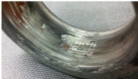
**Picture 2: Damage from bearing spinning on shaft.**
