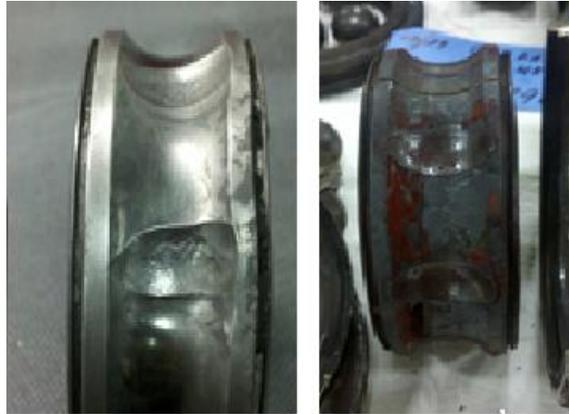
**Picture 3: Elliptical pockets and parasitic thrust damage.**
