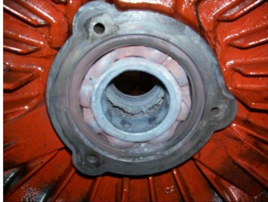
**Picture 1: Visual damage of radial preloading.**
