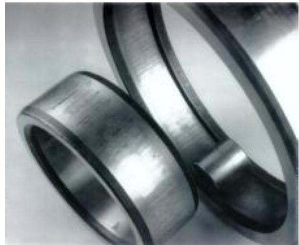
Figure 1. Example of an electric motor bearing that was subjected to vibration during stand-still. It concerned an auxiliary motor on a ship. The result is false brinelling marks (SKF Belgium).
