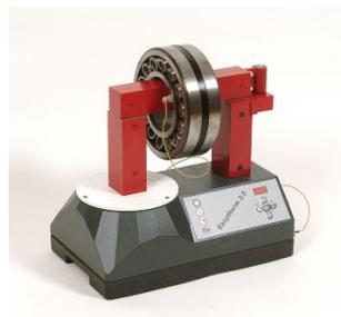
**Pic 2: Induction Heater (TM Easytherm 3.5)**
