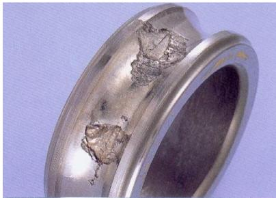
**Picture 1. Deep Groove Ball Bearing with flaking**
