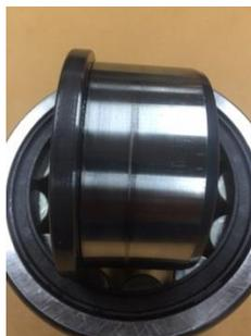
**Picture 2. Cylindrical Roller Bearing with skidding**
