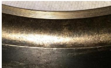
Picture 2: Bronze material embedded in raceway.
