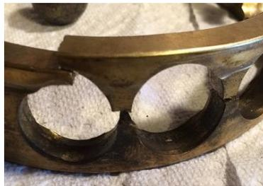
Picture 1: Worn and broken cage.
