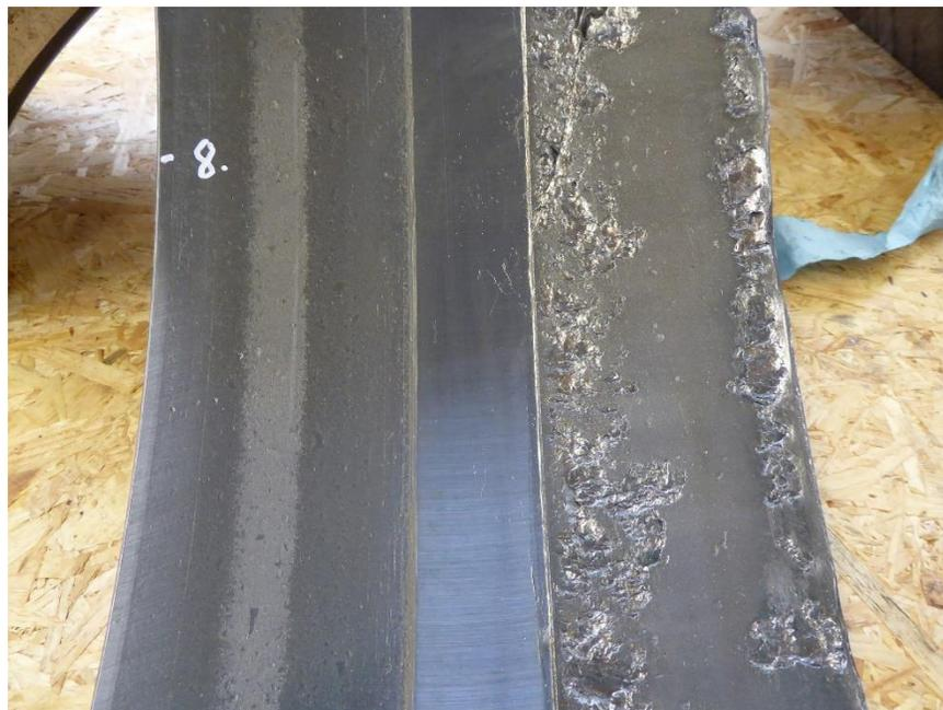
*Common main-shaft spherical roller bearing outer ring damage, upwind row left, downwind row*
