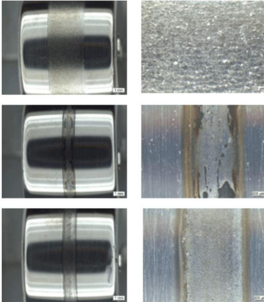
*MPR test cases one hour of operation after starvation. Steel on steel (top row), SKF NoWear on steel (2nd and 3rd row).*
