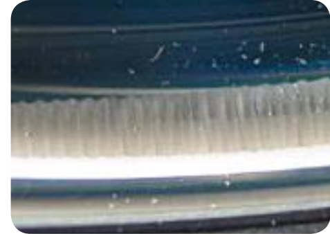
Fluting created by electrical arcing
