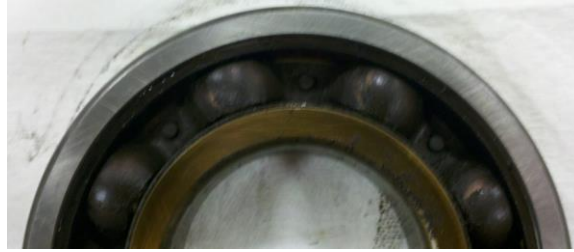
Picture 6: Discoloration of bearing
