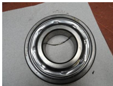
Pic 2: Collapsed shield, possible cause pressure from grease gun.
