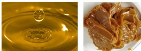
**Pic 2: Base oil (left) and Thickener (right.)**
