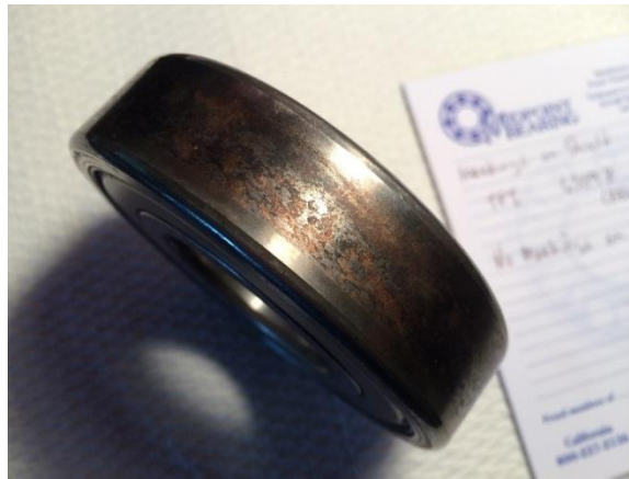
Pic 1: Fretting Corrosion on Outside Diameter
