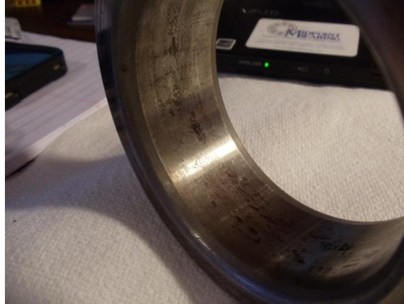
Pic. 2: Fretting Corrosion on Bore.
