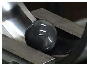
**Pic. 2: Ceramic ball in raceway, and resulting damage.**
