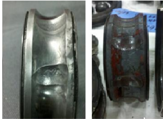
Picture 3: Elliptical pockets and parasitic thrust damage.
