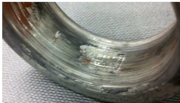
Picture 2: Damage from bearing spinning on shaft.
