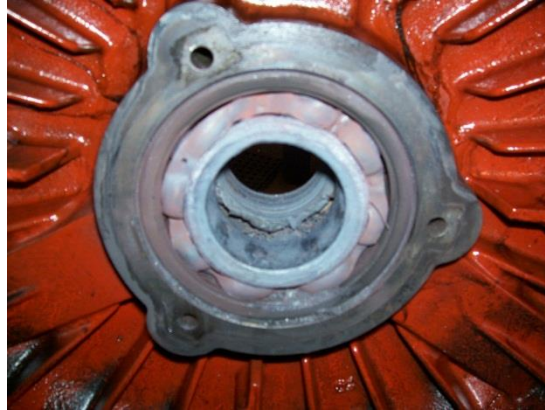
Picture 1: Visual damage of radial preloading.
