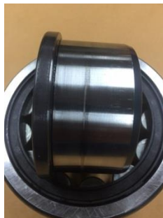
Picture 2. Cylindrical Roller Bearing with skidding
