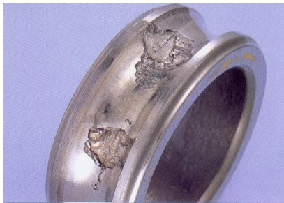
Picture 1. Deep Groove Ball Bearing with flaking
