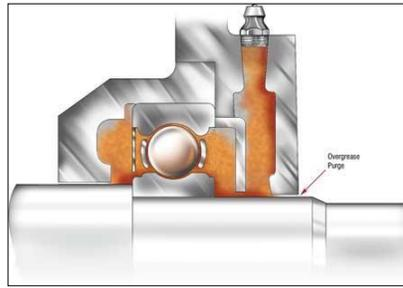
Fig 2: Grease shown in multiple cavities.
