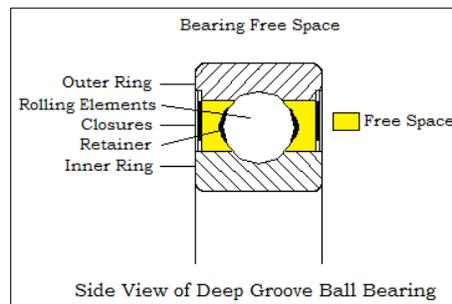
Fig 1: Representation of Bearing Free Space
